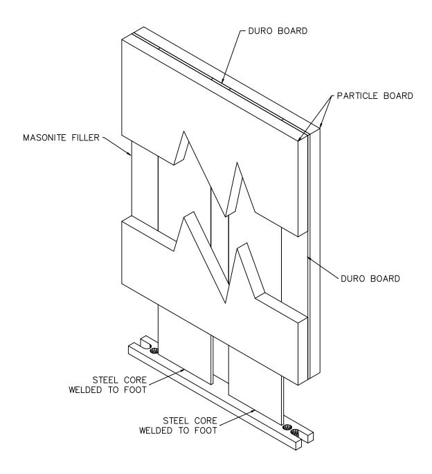
STEEL CORE SET UP IS THE SAME FOR OVERHEAD BRACED, FLOOR MOUNTED, CEILING HUNG & FLOOR TO CEILING
