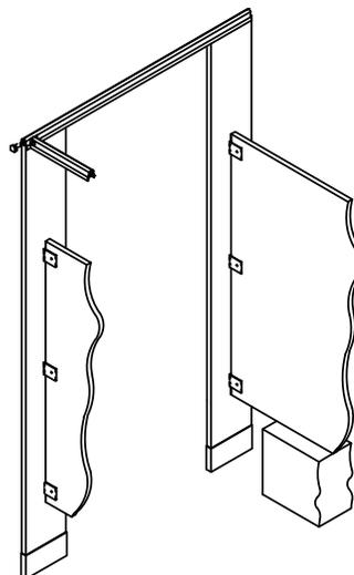
**FLOOR ANCHORED/OVERHEAD BRACED
